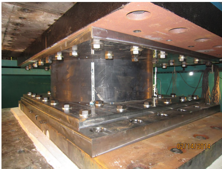
Figure 2 – The isolator under compression stiffness test.
