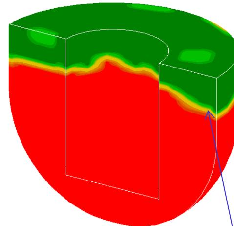
Another aspect that determine a further reduction of the impact force is the drug of the argon gas into the lead during the fluid motion causing the variation of lead density.
