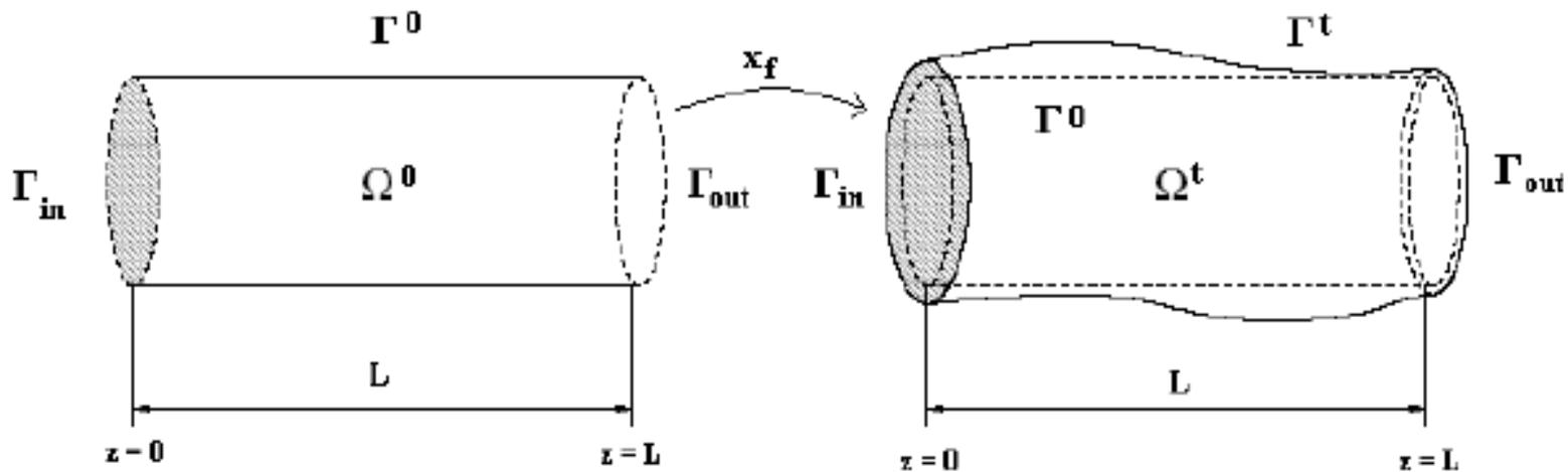
The new profile  $\Gamma^t$  (representing the liquid free surface motion induced by the FSI), from a mathematical point of view, is extremely complex and involves the speed and the pressure of the fluid, the displacement of the structure and the position of points in the domain  $\Omega^t$  at each instant  $t$ .
