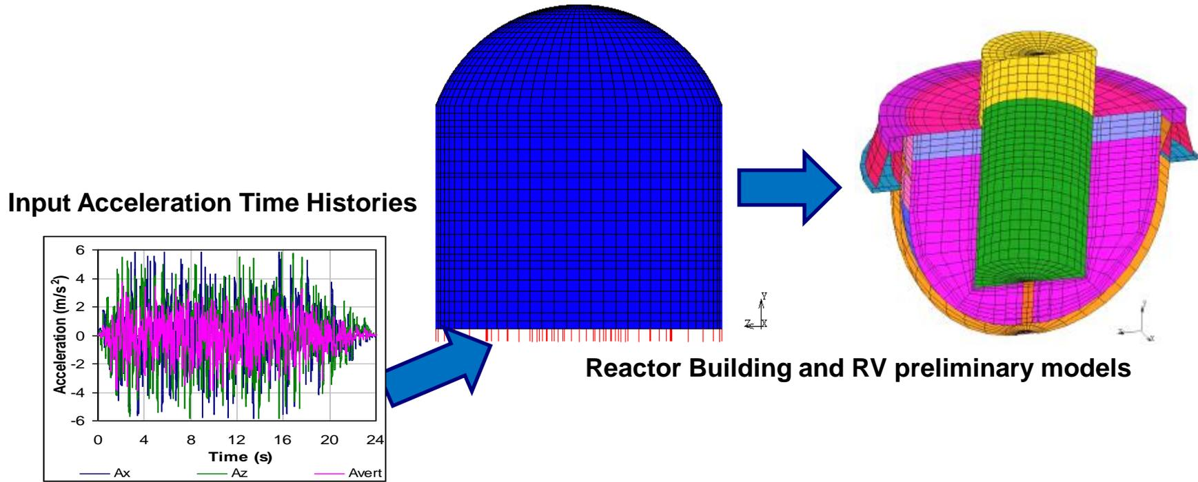
The input acceleration data were elaborated according to the updated R. G. US NRC 1.60 and 1.92, considering a 5% of critical damping value.
