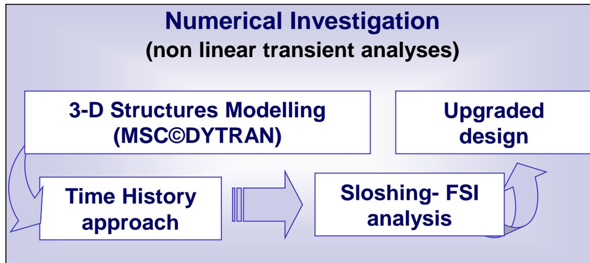
The solution of sloshing phenomenon will allow to determine the fluid motion, the hydrodynamic pressures and stresses of the RV and internals structures.
